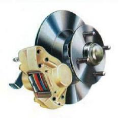
Powerful cars need powerful brakes and the power to stop is provided by Girling 11in. disc brakes in front, and wide, 9in. diameter drums at the rear. Together with the wide section sports tyres they give swift, smooth and skid-free retardation.
