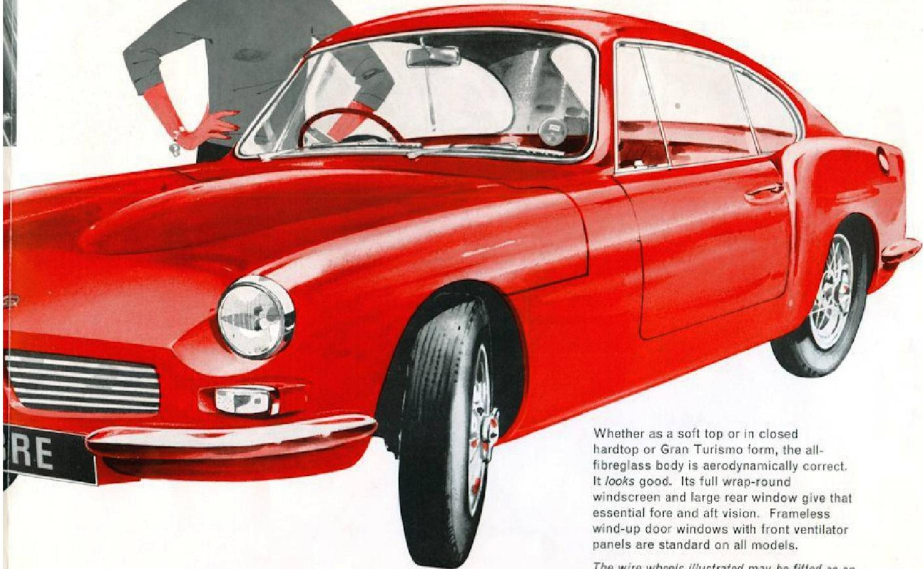
Whether as a soft top or in closed hardtop or Gran Turismo form, the all-fibreglass body is aerodynamically correct. It *looks* good. Its full wrap-round windscreen and large rear window give that essential fore and aft vision. Frameless wind-up door windows with front ventilator panels are standard on all models.
