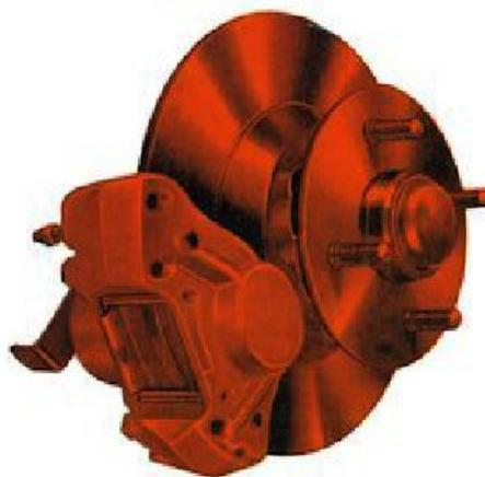
Powerful cars need powerful brakes and the power to stop is provided by Girling 10½ in. disc brakes in front, and wide, 9 in. diameter drums on the rear. Together with the wide section sports tyres they give swift, smooth and skid-free retardation.
